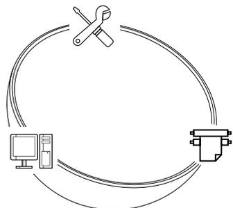
In a business centre, where separate businesses run on different phases of the building supply. If one company runs some large loads (eg: printing equipment), another runs small loads (eg: computers) and a third only employs assembly workers with no electrical load, then the building electrical system can be unbalanced. One business may be experiencing low or high voltages, due to another business, through no fault of its own.
