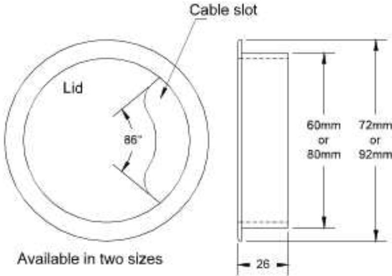
The FLOOR GROMMET is a simple but effective circular floor port allowing access to under floor cables and sockets. Easily installed in most types of raised floors and designed to withstand normal office loadings.
