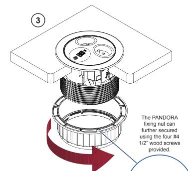
NOTE: The power cable to the Pandora unit must arranged/secured below the fixing surface so as not to restrict the rotating mechanism.
