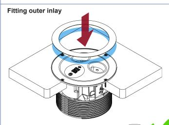
To fit the outer inlay, remove the VHB tape cover, align with the outer grommet, and then press down firmly.
